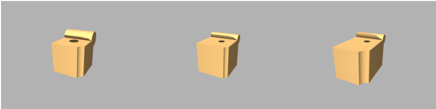
Fig. 1. Illustration of a parameterized template FRep model: a model is built with FRep in a constructive way with abstract parameters that can be tuned to satisfy some modeling criteria
