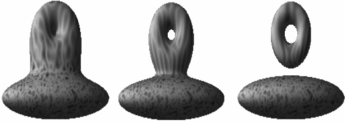
Fig. 8. Changing the area of influence and \vartheta . The Z function is defined as a FRep tree, composed of an intersection of a block and a torus. From left to right, the \vartheta parameter in the \tilde{Z} function is defined as \vartheta < 1 , \vartheta = 1 and \vartheta > 1 .
