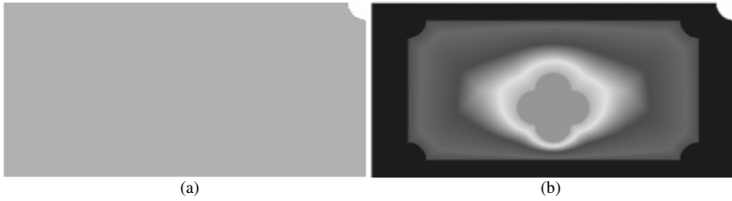
Fig. 6. Two-dimensional CAD part. (a) Geometry of the CAD part defined by an FRep model. (b) Three different material regions (outer black: material 1, inner constant grey: material 2, grey gradient: functionally graded material).
