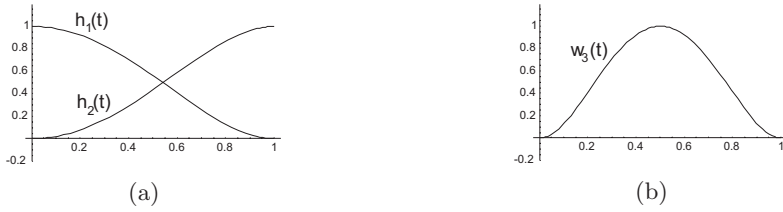
Fig. 10. (a) Weighting functions h_1 and h_2 . (b) The weighting function w_3 has the maximum in the middle.
