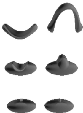
Fig. 6. Influence of the parameter r in the definition of the space mapping. An ellipsoid is deformed using space mapping with one control point displaced towards the inside of the object (left column) and outside (right column) with three different values of the parameter r .
