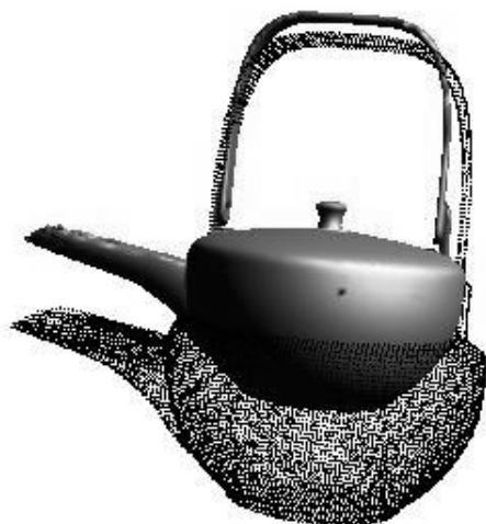
Fig. 5. Local minimum effect: result of the fitting with a local method starting with initial parameters far from the global optimum. The point-set for the sake pot is also displayed for comparison.
